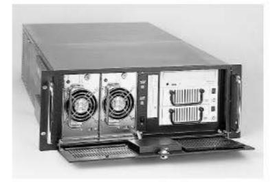
The IPC-623 features a front-accessible hot-swap redundant 300 W power supply with on/off key lock for easy maintenance and replacement.
